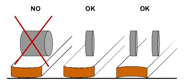
Figure 1. Recommended infeed rollers to avoid cracking of the boards.
